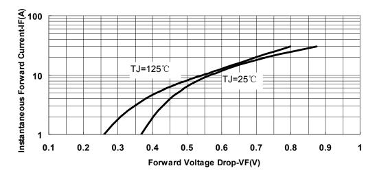
Fig.3-Typical Instantaneous Forward Voltage Characteristics
