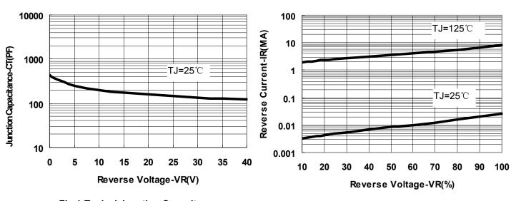
Fig.1-Typical Junction Capacitance
